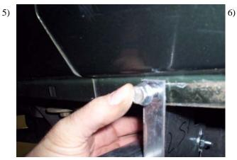
Insert a 5/16" flange bolt trough pinch weld and BT68 and tighten with a 5/16" flanged nut. Tighten all nuts and bolts (BT68 show on outside of pinch weld for picture purpose only bracket goes on inside of pinch weld)
