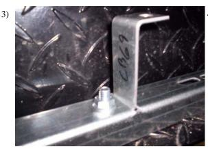
Attach BT68 to each CB bracket with a 5/16" flanged nut and bolt as shown. (**Different BT bracket shown**)
