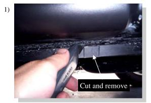
Measure from front wheel well back and make a mark at 10-1/2", 33-1/2", 55". At each mark, remove about a 1-1/4" wide piece of the cladding covering the pinch weld.
