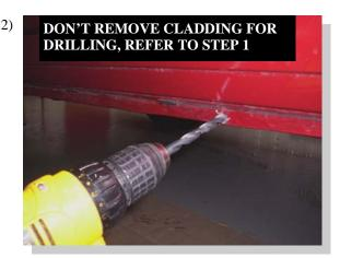
At each of the locations from step one, drill a 5/16" hole through the pinch weld. (**Different vehicle shown**)
