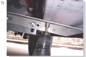
Set the board on the brackets. Make sure the board is centered between the wheel wells and is aligned evenly down the side of the vehicle Attach the board to the brackets with 3/4" long self drilling screws. Don't attach lip of board to vehicle.
