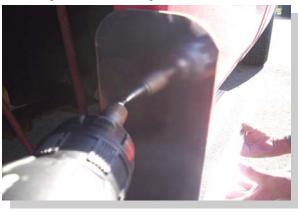
Use one self drilling screw to attach the stone guard to the fender lip. Make sure the board is level, then use remaining 2 screws to finish attaching stone guard to fender lip.
