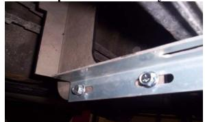
Std cab: Attach 3124F at Dr rear and pass front location, attach 3124L at Dr front and pass rear location using 5/16" flanged nut and bolts as shown.
