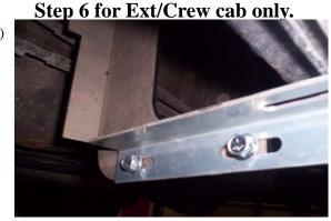
Ext/Crew cab: Attach 3124F at Dr rear/middle, pass front/middle location, attach 3124L at Dr front and pass rear location using 5/16" flanged nut and bolts as shown.
