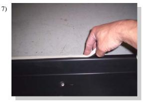
Apply foam tape to the top lip of the board. Apply the step tread also at this time.
