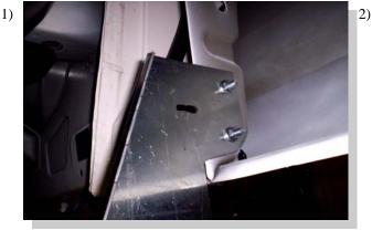
Attach the FL152 bracket to the front bed side-wall support using 5/16" bolts and nuts.
