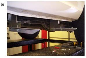
Attach a 3124J angle bracket (the shorter one) to FL152 3124G to FL206D/P with 5/16" bolts and nuts. Snug but do not tighten at this time.
