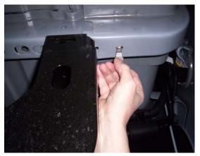
Insert 8mm pull nut, turn bracket back to original position, and install 8mm bolt, flat washer, and lock washer. Tighten 12mm flanged bolt.
