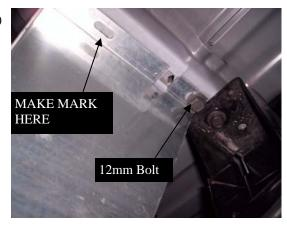
In front of rear wheel, above front leaf spring shackle on the bed cross member, attach FL206D/P with 12mm flanged bolt. Just snug bolt. Make a mark in the center of the slot so you can turn bracket and drill a 1/2" hole.
