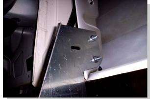
Attach the FL185 bracket to the front bed sidewall support using 5/16" bolts and nuts.
