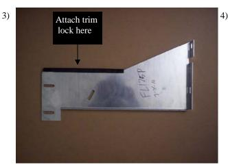
Cut trim lock to 11" and attach as shown in **Fig 3.** (**DIFFERENT BRKT SHOWN**)
