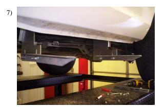
Attach a 3124F angle bracket to the FL185 and FL206D/P with 5/16" bolts and nuts. Snug but do not tighten at this time.
