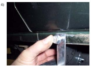
Insert a 5/16 flanged bolt through pinch weld and FL205 and tighten with 5/16" flanged nut. Now tighten 8mm nuts.
