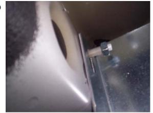
Install FL205 at the marks you made on pinch weld by inserting vehicle stud through slot in FL205 and attach with two 8mm nuts. Snug but don't tighten yet.
