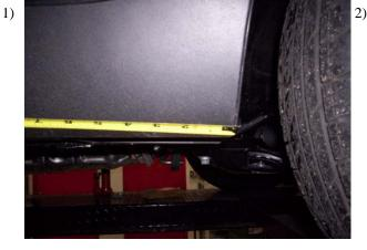
Measure from front wheel well back making a mark on the pinch weld at 16" 37" 67" for King cab and 16" 37" 67" 79" for Crew cab.
