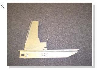
Attach one 3124F to FL205 using 5/16 bolts and nuts. Snug but do not tighten. (**DIFFERENT BRACKET SHOWN**)
