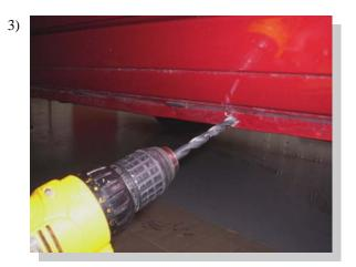
Drill a 5/16" hole in pinch weld at pre-marked location, to insert a 5/16" flanged bolt through pinch weld and FL205.
