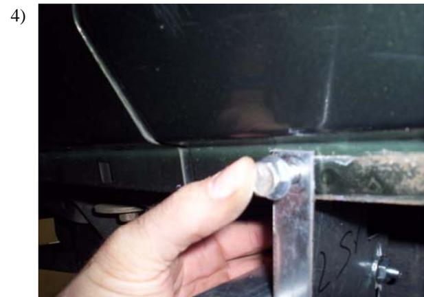
Drill a 5/16" hole in pinch weld at pre-marked location, to insert a 5/16" flanged bolt through pinch weld and FL204.
