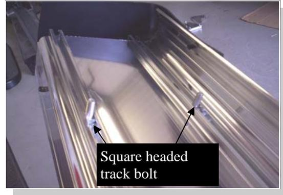
For Aluminum Boards: Insert one square headed track bolt into both tracks for each bracket.
