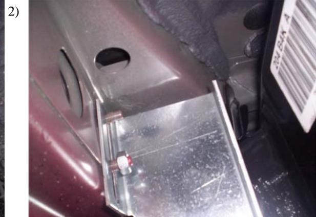
Measure from front wheel well back making a mark on the pinch weld at 15" 35" 62" for King cab and 15" 35" 67" for Crew cab.
