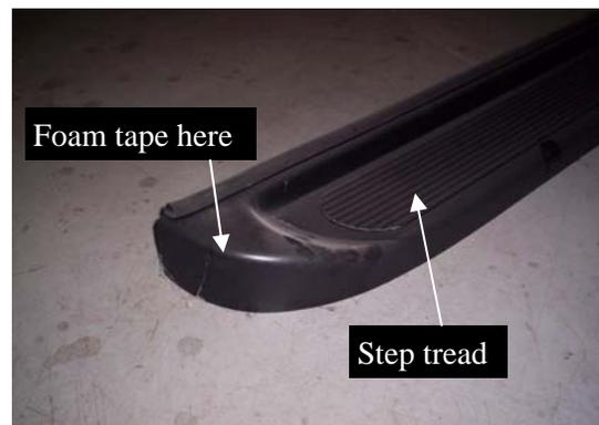
On ABS boards only, apply foam tape and step tread as shown in picture. Center step tread between the ends of the board and keep close to outside edge.
