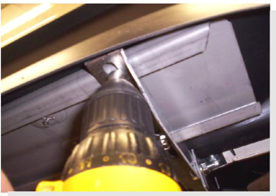
For Molded Boards: Position board where you want it. Install self tapping bolts through bracket into the shoulder of the steel channel on the bottom of the board.
