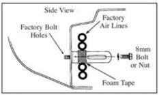
2.On passenger side with air and heat lines, wrap AS02 angled strap with foam tape so that lines are protected. Attach AS02 with 8mm bolts or nut to factory bolt holes on passenger and driver sides. Do not tighten at this time.
