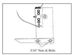
Attach 3124F step support to flat plate using two 5/16" nuts and bolts. Do not tighten at this time.
