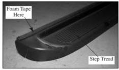
7.On ABS boards only, apply foam tape and step tread as shown in picture. Center step tread between the ends of the board and keep close to outside edge.
