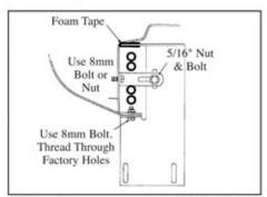
3. Place foam tape at top of FL102 flat plate. Bolt to AS02 then to pinch weld with 8mm bolts. Note: top of flat plate must hit rocker panel. Tighten to AS02 and 8mm bolt before tightening to pinch weld.
