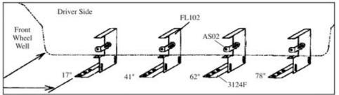
1.Measure from front wheel well, back 17", 41", 62", and 78". Mark these bracket locations. Note: Factory holes should be close to these measurements; use factory holes only.
