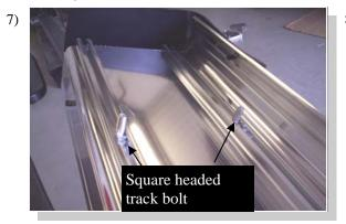
For Aluminum Boards: Insert one square headed track bolt into both tracks for each bracket.
