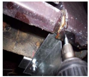
Insert a self tapping bolt through vehicle body lip into FL20 and tighten.
