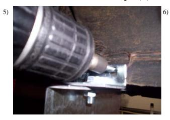
Insert a self tapping bolt through each hole in BT07 into the pinch weld and tighten bolts, next tighten 5/16" flanged nut and bolt.
