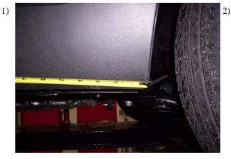
Measure from front wheel well back making a mark on the pinch weld at 13"& 36" for STD cab, 13", 40" & 66" for EXT cab.
