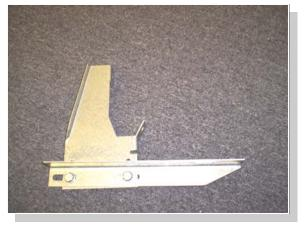
Attach one 3124F to FL09 using 5/16 bolts and nuts. Snug but do not tighten. (**DIFFERENT BRACKET SHOWN**)
