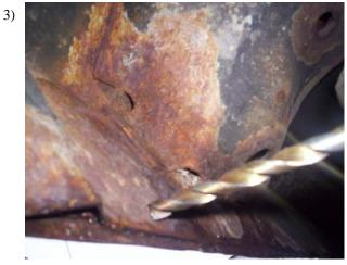
Hold FL09 up at the location where the marks were made. Make a mark in the bottom hole, then drill a 5/16" hole through the pinch weld where you made the mark. Insert a 5/16" flanged bolt through pinch weld and bracket and tighten with 5/16" flanged nut.
