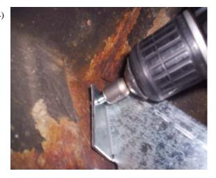
Attach top of FL09 by inserting a self tapping bolt through hole in bracket and into vehicle's body and tighten.
