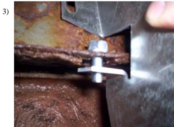
Install BRKKT assembly to vehicle by attaching FL47 at 13" measurement and FL46D/P (D-Driver side, P-Passenger side) at the remaining measurements. Insert 5/16" flanged bolt through factory hole in pinch weld and through brackets and tighten with 5/16" flanged nut. If there is no hole drill a 5/16" hole through pinch weld.
