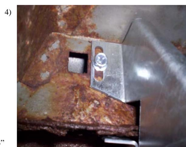
Insert a 5/16" flanged bolt through bracket and attach to clip nut. Some vehicles you will not have this hole, so you will have to use a self tapping bolt.
