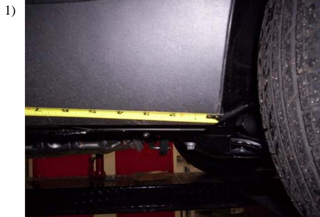
Measure from front wheel well back making a mark on the pinch weld at 13" & 36.5" for Std cab, 13", 36.5" & 47.5" for Ext cab, 13", 44" & 71" Super Crew Cab. 13" 44" 60" 78"
