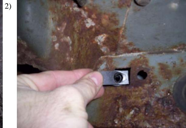
Insert clip nut into body holes at all bracket locations.
