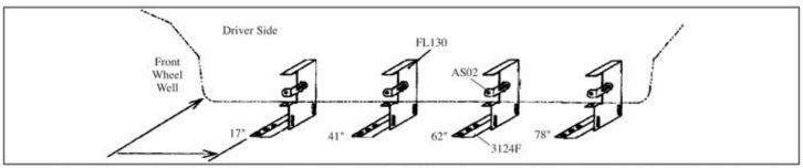
Measure from front wheel well, back 17", 41", 62", and 78". Mark these bracket locations. Note: Factory holes should be close
