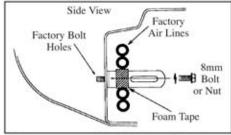
2.On passenger side with air and heat lines, wrap AS02 angled strap with foam tape so that lines are protected. Attach AS02 with 8mm bolts or nut to factory bolt holes on passenger and driver sides. Do not tighten at this time.
