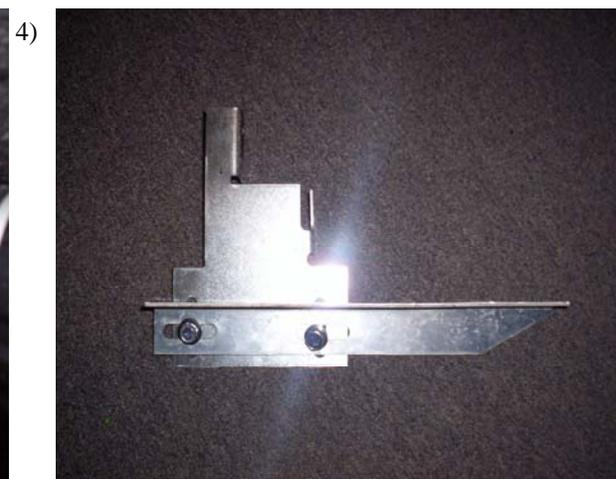
Attach one 3124F to FL202 using 5/16 bolts and nuts. Snug but do not tighten.
