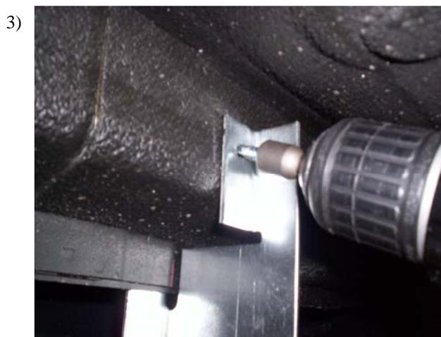
Install FL202 by inserting a 5/16" flanged bolt through the hole you drilled in the pinch weld and tighten with 5/16 flanged nut. Next insert self tapping screw into 1/4 hole in top side of bracket.
