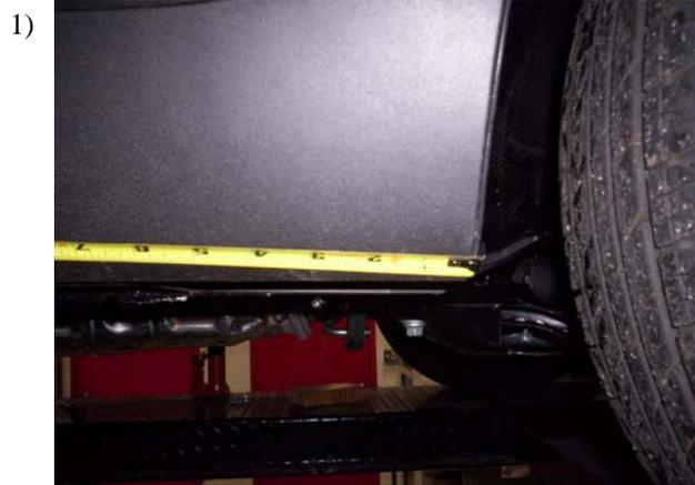
Measure from front wheel well towards the rear and make a mark on pinch weld at 14" 31" 44" 59". At these locations you will have to notch the plastic body molding so you can drill a 5/16" hole through pinch weld.
