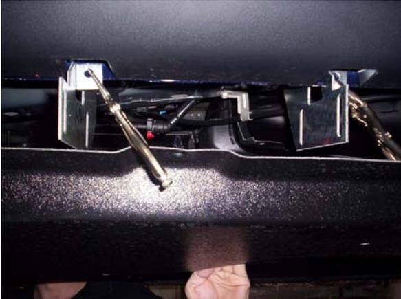
After all FL202's are installed you will have to cut a slit in the splash shield at the 44" bracket location, so you can reinstall the splash shield around the bracket.
