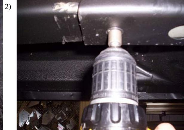
Remove plastic splash shield on the under body, by removing all the 10mm bolts holding in place. There is one on both sides of vehicle. Save bolts and splash shields for reinstall.
