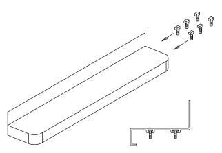
FOR EACH BRACKET SLIDE ONE 1/4" X 5/8" SQUARE HEAD SCREW INTO EACH TRACK,
