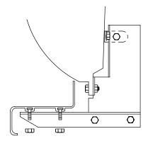
SECURE BOARD TO BRACKET WITH 1/4" NUTS
