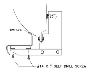
FOR PLASTIC BOARDS, APPLY FOAM TAPE AND STEP TREAD TO BOARD. ATTACH THE BOARD TO THE BRACKETS WITH SELF DRILLING SCREWS.
