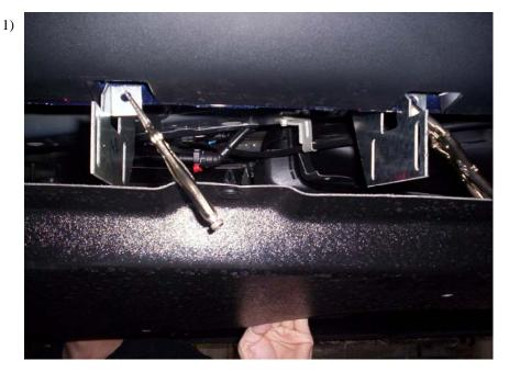
Start by removing the splash shield under the vehicle, on both sides, keeping all push pins and bolts for shield re-installation. Install brackets as per instruction sheet IN348. After brackets are installed and before installing board, hold splash shield up in place and make a mark on shield where each bracket is. You will have to cut a slit in the shield at each bracket location to install it back in place.
