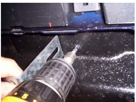
After you reinstalled splash shield, install a self tapping screw on each side of the bracket where you cut a slit in the shield by the pinch weld.
