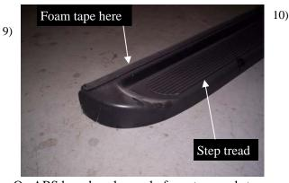
On ABS boards only, apply foam tape and step tread as shown in picture. Center step tread between the ends of the board and keep close to outside edge..
