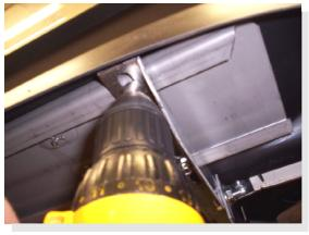
Position board where you want it. Install self taping bolts through bracket into the shoulder of the steel channel on the bottom of the board.
