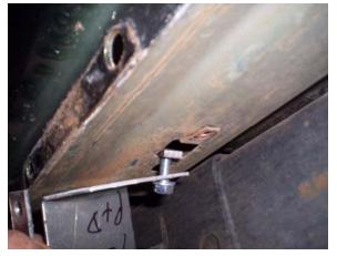
At 19" measurement insert 5/16" flanged bolt through FL157P to flat retaining nut. Insert retaining nut into hole in under body. Next insert 5/16" flanged bolt through bracket and pinch weld as in step #2. Tighten all bolts for this bracket.
