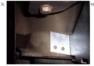
Next install self tapping bolts through top of bracket into under body. Now tighten 5/16" flanged nut and bolt for this bracket.
