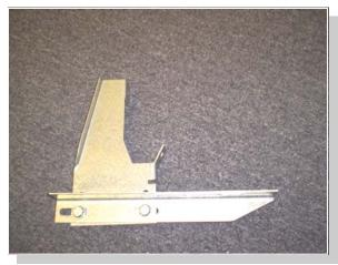
Attach one 3124F to FL157D/P using 5/16 bolts and nuts. Snug but do not tighten. (**DIFFERENT BRACKET SHOWN**)
