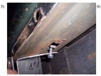
At 43" measurement insert 5/16" flanged bolt through FL157D to flat retaining nut. Insert retaining nut into hole in under body. Next insert 5/16" flanged bolt through bracket and pinch weld as in step #2. Tighten all bolts for this bracket.
