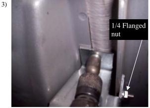
Next install self tapping bolts through top of FL195D/P and FL197 into under body. Now tighten 1/4" flanged nut for these brackets.
