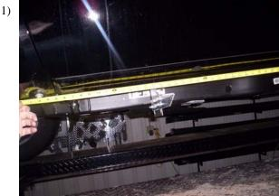
Measure from front wheel well towards the rear and make a mark on pinch weld at 16" 36" and 58". There should be a hole at these locations.
