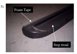
Apply foam tape and step tread as shown in picture. Center step tread between the ends of the board and keep close to outside edge.
