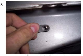
At measurement 36" install FL196D/P by first installing a pull nut into oblong hole in underbody, then insert 1/4" carriage bolt through hole in pinch weld and through bracket, and attach with 1/4" flanged nut. Insert 8mm bolt through bracket into pull nut. Install self tapping bolt through top of bracket into under body. Tighten all nuts and bolts.
