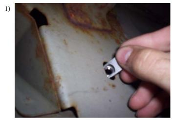
Measure back from front wheel well on driver side 69" and make mark on pinch weld. Above the rear A/C lines there is a slot in the body. Insert pull nut into slot. Make a mark on the pinch weld and drill a 5/16" hole. If no slot continue to next step.
