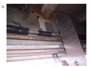
Attach FL199 by inserting either 8mm bolt through top hole in FL199 to pull nut, or if no hole for pull nut use self tapping bolt. Next insert 5/16 flanged bolt through hole in pinch weld and through slot in FL199 and tighten. Follow the rest of the steps in the other instruction sheet for board installation.
