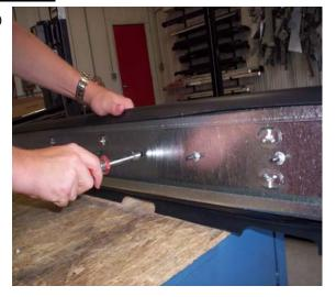
Tighten using 7/16 nut to step pad post. Just snug nuts do not over tighten.
