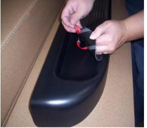
Position step tread where you want it. Then holding step tread in place remove adhesive cover one row at a time and press firmly to hold in place.
