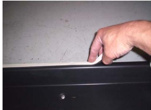
Apply foam tape to the top lip of the board. Apply the step tread also at this time.
