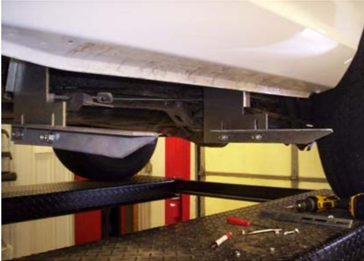
Attach a 3124J angle bracket (the shorter one) to FL152 3124G to FL175D/P with 5/16" bolts and nuts. Snug but do not tighten at this time.
