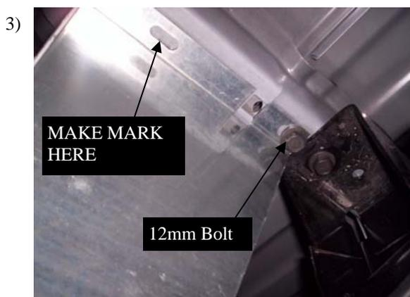
In front of rear wheel, above front leaf spring shackle on the bed cross member, attach FL175D/P with 12mm flanged bolt. Just snug bolt. Make a mark in the center of the slot so you can turn bracket and drill a 1/2" hole.
