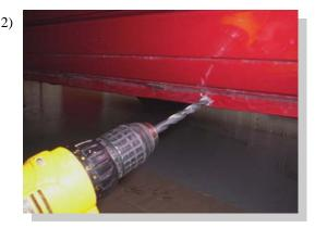
At each of the locations from step one, drill a 5/16" hole through the pinch weld, if no factory hole is present.
