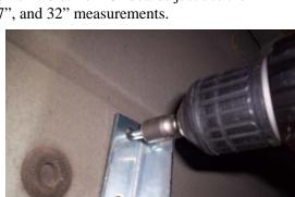
Attach 3124F to FL105 with two 5/16 nuts and bolts, snug but do not tighten yet. Attach brackets to vehicle by inserting the 5/16" bolt and nut through the pinch weld. Then install the self tapping bolts through the brackets into the body.
