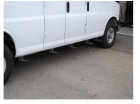
Measure from front wheel well back and make a mark at: 7",32",64",92" along the pinch weld. For 40" boards just use the 7", and 32" measurements.
