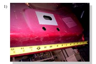
Measure from front wheel well back and make a mark at: 10",25",47",67",78" along the pinch weld.
