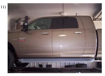
Level the board and tighten all bolts. Repeat steps for the opposite side. (NOTICE SHOWN WITH FIBERGLASS BOARD)
