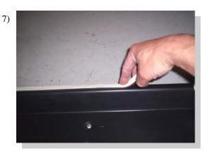
Apply foam tape to top edge of the board. Apply the logo and step tread to clean and dry running board. Allow tread to cure (no inclement weather for 48 hours).
