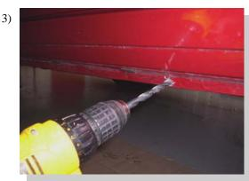
At each of the locations from step one, drill a 5/16° hole through the pinch weld.
