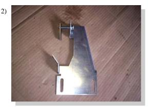
Assemble brackets as shown using one 5/16" bolt and steel retaining nut.
