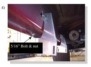
Attach brackets to vehicle by inserting the retaining nut in the factory ob-round hole and using one 5/16" bolt and nut through the pinch weld.
