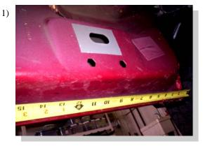
Measure from front wheel well back and make a mark at : 10",25",47",67",78" along the pinch weld.
