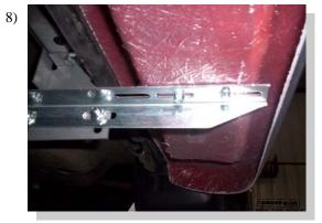
Place the board on the brackets and align up on the vehicle. There is a driver and a passenger side board. Attach to the brackets using  $#14 \times 3/4$ " long self drilling screws, making sure you are drilling through steel mounting pad on under side of board.
