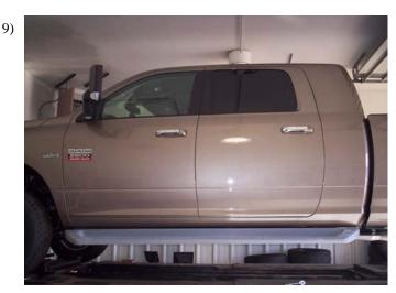
Level the board and tighten all bolts. Repeat steps for the opposite side.
