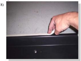
Apply foam tape to the top lip of the board. Apply the step tread and logo also at this time.
