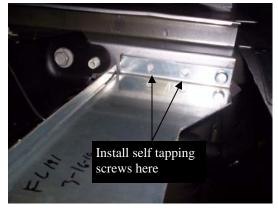
Attach the FL181 bracket to the front bed cross member support, using 5/16" bolt, as shown in **Fig. 2.** Next install self tapping screws into the other holes in the bracket to the cross member.
