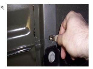
In front of rear wheel, above front leaf spring shackle, on the bed cross member, install 8mm pull nut as in **Fig 5.**
