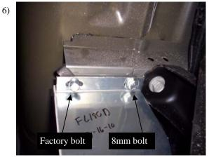
Install FL180 D & P using factory bolt you removed in step 4 and 8mm bolt and washers, as in **Fig. 6.**
