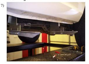
Attach a 3124F angle bracket to the FL181 and the 3124G (the longer angle) to the FL180D & P with 5/16" bolts and nuts. Snug but do not tighten at this time.
