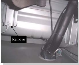
In front of rear wheel, above front leaf spring shackle, on the bed cross member, remove factory bolt holding fender brace. Save bolt you will need it later.
