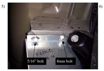
Install FL180D & P using 5/16" flanged bolt and 8mm bolt and washers, as in **Fig. 5.**
