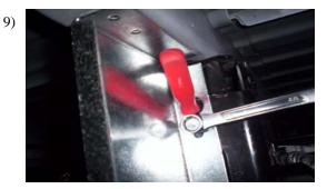
Once bracket is straight tighten upper bolt, you may need to insert a small screwdriver into slot as shown **FIG # 9** to keep nut from turning. Then tighten lower bolt.
