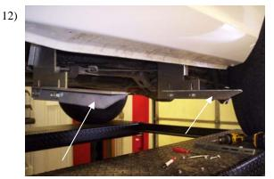
You are now ready to attach angles to installed brackets using 5/16" bolts and nuts, snug for now. The longest angle should be attached to the front FL152 and the shortest to the rear FL172. If you are having trouble lining up the box board with the cab board, you can change these angles around for a better line up if needed.
