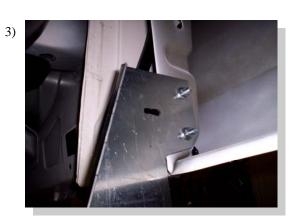
Attach the FL152 bracket to the box sidewall support using 5/16" bolts and nuts.
