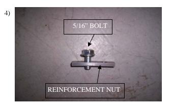
Thread 5/16" bolt into the hole that's closest to center as shown in **FIG# 4.**
