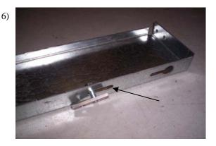
Insert 5/16" bolt through lower slot on FL172, Then thread bolt into center hole of reinforcement nut as shown above **FIG# 6**
