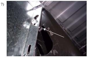
Take FL172 with nut attached as in step 6, and insert the large keyhole slot over the bolt head **FIG** # **5**, angling the FL172 to allow access to rear of bolt through large frame support slot. You will need to reach through large slot and hold the bolt from falling into frame support. Push up on bracket when head is through key hole slot.
