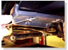
Remove the plastic edge protector on the front edge of the box. To remove, use a small screw driver to pull out the push pin. Remove and discard.
