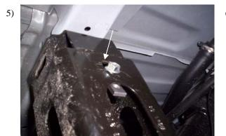
In front of the rear wheel you'll see a frame support that the bed cross member bolts to. Install bolt head with reinforcement nut through top slot as shown above **FIG# 5**
