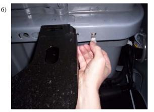
Insert 8mm pull nut, turn bracket back to original position, and install 8mm bolt, flat washer, and lock washer. Tighten 12mm flanged bolt.
