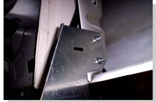
Attach the FL152 bracket to the front bed sidewall support using 5/16" bolts and nuts.
