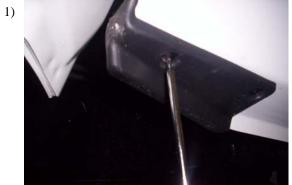
Remove the plastic edge protector on the front edge of the box. To remove, use a small screw driver to pull out the push pin. Remove and discard.
