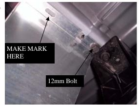
In front of rear wheel, above front leaf spring shackle on the bed cross member, attach FL175D/P with 12mm flanged bolt. Just snug bolt. Make a mark in the center of the slot so you can turn bracket and drill a 1/2" hole.
