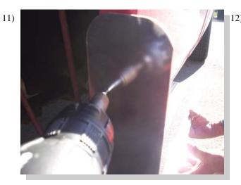
Use one self drilling screw to attach the stone guard to the fender lip. Make sure the board is level. Use remaining 2 screws to finish attaching stone guard to fender lip.
