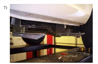
Attach a 3124F angle bracket to the FL152 and FL175D/P with 5/16" bolts and nuts. Snug but do not tighten at this time.
