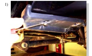
Remove the plastic edge protector on the front edge of the box. To remove, use a small screw driver to pull out the push pin. Remove and discard.
