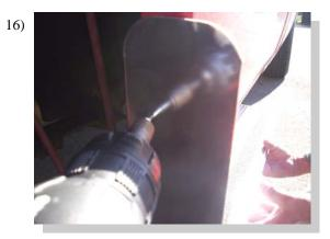
Using self drilling screws attach the stone guard to the fender lip. Make sure the board is level.
