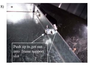
Once the FL172 is pushed up you'll need to push the lower bolt up in the slot and turn the reinforcement nut to fit into large slot in frame support. Make sure reinforcement nut is catching frame support, straighten and push up bracket then snug lower bolt.
