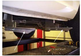
You are now ready to attach angles to installed brackets using 5/16" bolts and nuts, snug for now. The longest angle should be attached to the front FL152 and the shortest to the rear FL172. If you are having trouble lining up the box board with the cab board, you can change these angles around for a better line up if needed.
