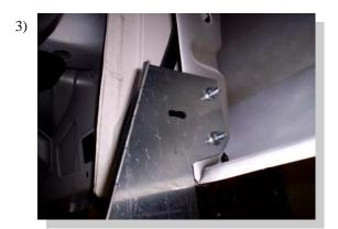
Attach the FL152 bracket to the box sidewall support using 5/16" bolts and nuts.
