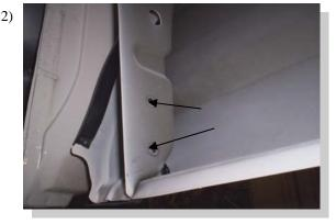
Locate the holes in the front bed sidewall support.
