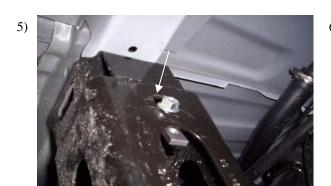
In front of the rear wheel you'll see a frame support that the bed cross member bolts to. Install bolt head with reinforcement nut through top slot as shown above **FIG# 5**
