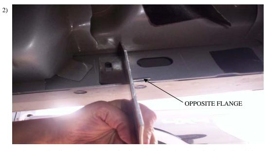
In the <u>center location only</u>, the brackets in Fig.1 are to be used as shown in Fig#2. They will line up with the factory hole in your truck.
