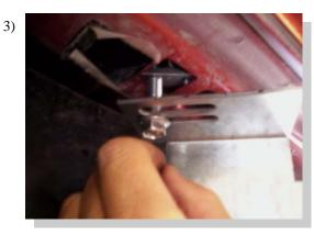
You will need to insert reinforcement nut into hole under vehicle at the the measured locations as stated in Fig. 1
