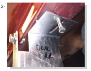
Attach bracket with 1 slot to vehicle at measured location 62". The rear locations use an 8mm bolt and a factory threaded hole. Straighten bracket and bolt through pinch weld.
