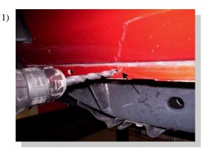
The bracket locations should be measured from front of <u>pinch weld</u> to approx. locations. The front 12", middle 36 and rear at 62".You may need to drill for clearance.
