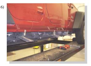
Attach channels to the body mounting Brackets you just installed, hand tighten making sure to keep channels level to body.
