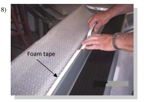
Apply foam tape to rear lip of board where it meets up with the vehicle. Apply step tread and logo now also. (Board in photo is not of the Lexus board)
