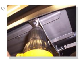
Place board on the 3124F brackets, position board so it fits snug up against the vehicle and is level. Attach with 3/4" long self drilling screws through slots in the 3124F's into the steel plate under the board. Tighten bolts holding the 3124Fs to the flat brackets.
