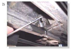
At measured locations it will be necessary to trim the plastic covers. Carefully remove the retaining clip and open cover. Keep the clip to reinstall after trimming.
