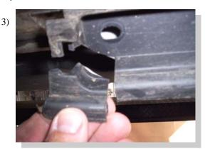
Trim the plastic cover enough to clear the bolt head. Each cover may need to be trimmed a little differently to work. Close cover and install the clips removed in step two.
