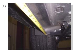
Measuring from the front wheel well, measure towards the rear of the vehicle. At locations 13", 38-1/2" and 61" (13", 40-1/2" and 59-3/4" Passenger Side), make a mark on the pinch weld.
