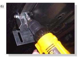
Attach brackets at proper locations using a 5/16" bolt and nut and one self drilling screw as shown .
