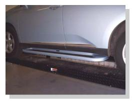
Repeat steps for opposite side being sure to use the noted dimensions in step one. Dimensions for each side are different. Use 67076D board on driver side and 67076P on passenger side.
