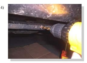
At each measured location drill a 23/64" hole through the pinch weld .
