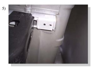
Locate the bed floor support in front of the rear wheel. This is where the brackets will attach.
