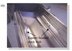
Insert one square headed track bolt into each track on the bottom of the board for each bracket.
