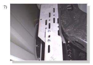
Attach FL74 to FL73 in the holes shown with 5/16" bolts and nuts.
