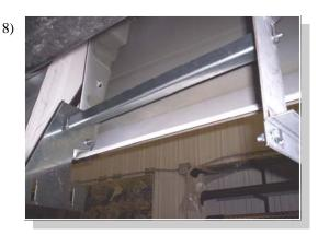
Attach CH07 brace between the two brackets with 5/16" bolts and nuts.
