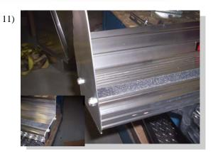
Attach stone guard and end cap to running board using 3/8" self threading bolts.
