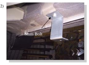
Attach the front two "Z" brackets to factory holes with 8mm bolts. The rear "Z" bracket will attach with supplied bolt/wire and nut.
