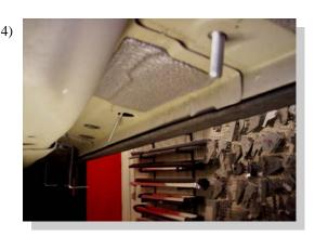
Photo of rear bolt after being installed. NOTE: It may be easier to install by putting a slight bend in the wire.
