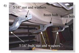
Attach bracket marked M-R to center location and bracket marked F to front location as shown. Tighten all hardware.
