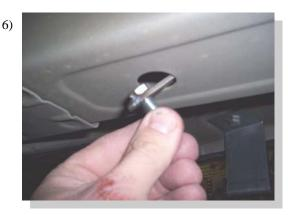
Insert bolt with welded tab into the forward hole in the frame for the front bracket to mount to.
