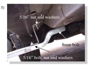
Attach bracket marked M-R and "Z" bracket to vehicle as shown at the rear location.
