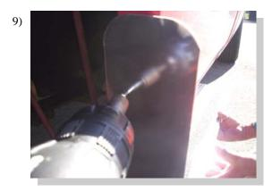
Using self drilling screws attach the stone guard to the fender lip. Make sure the board is level.
