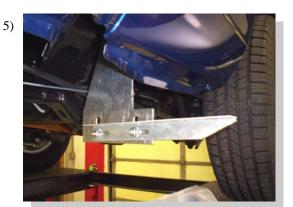
Attach a 3124F angle bracket to the FL152 with 5/16" bolts and nuts. Snug but do not tighten at this time.
