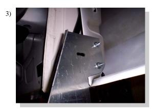
Attach the FL152 bracket to the sidewall support using 5/16" bolts and nuts.
