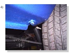
Remove the factory fender brace bolt but do not discard. This will be re-installed to hold the board. IN391
