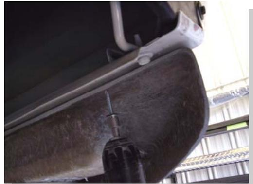
Using the longer self drilling screws with the rubber washer, attach the board to the truck bed through the lip of the bottom lip of the board..
