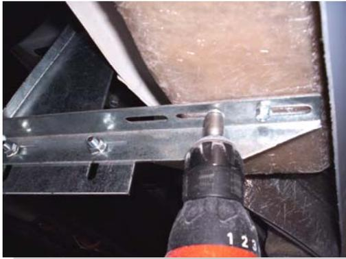
Align the board on the brackets with the cab boards and attach with self drilling screws..
