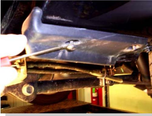
Remove the plastic edge protector on the front edge of the box. To remove, use a small screw driver to pull out the push pin. Remove and discard.
