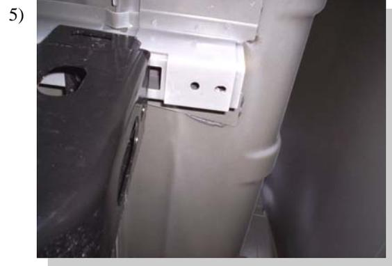
Locate the bed floor support in front of the rear wheel. This is where the brackets will attach.
