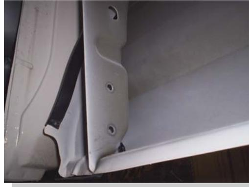
Locate the holes in the front bed sidewall support.
