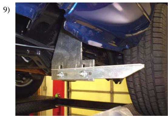
Attach one 3124F to front bracket and one 3124J to the rear bracket with 5/16" bolts and nuts. Snug but do not tighten.
