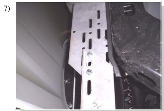
Attach FL74 to FL73 in the holes shown with 5/16" bolts and nuts.
