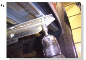
For ABS plastic boards, place on brackets and align on truck. Using self drilling screws attach the board to the brackets.
