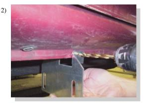
At each of the locations from step one, hold a bracket in place and drill a 5/16" hole through the pinch weld where the bracket will attach.
