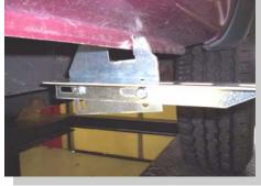
Attach 3124F angle support to FL153 flat bracket with 5/16 bolts and nuts. Snug but do not tighten.
