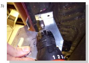
Attach the bracket with a 5/16" bolt and nut through the bracket and drilled hole. Use one self drilling screw to attach to under body. Tighten all bolts.
