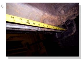
Measure from front wheel well back and make a mark at : Std Cab-13" & 38" Ext Cab-13", 34" & 56" Crew Cab—13", 31", 49" & 69"
