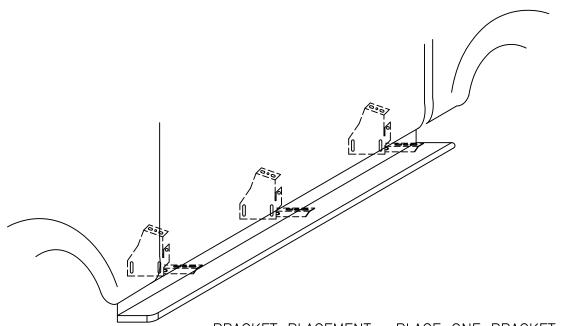
BRACKET PLACEMENT: PLACE ONE BRACKET IN THE CENTER AND THE THE OTHER TWO BRACKETS EVENLY SPACED OUT TO SUPPORT THE BOARD.
