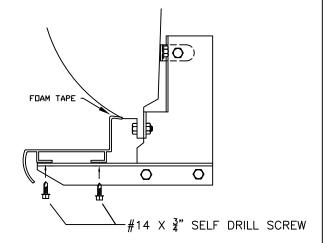
FOR PLASTIC BOARDS, APPLY FOAM TAPE AND STEP TREAD TO BOARD. ATTACH THE BOARD TO THE BRACKETS WITH SELF DRILLING SCREWS.
