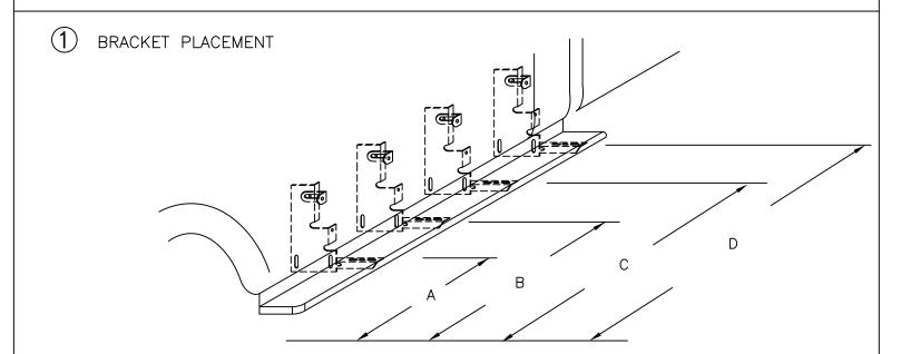
MEASURE FROM FRONT WHEEL WELL TO BRACKET LOCATION MARK THIS DIMENSION ON THE PINCH WELD
