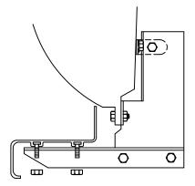
SECURE BOARD TO BRACKET WITH 1/4" NUTS
