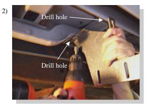
At each of the locations from step one, hold a bracket in place and drill a 23/64" hole through the cab supports where the bracket will attach.
