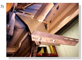
Attach the bracket with a 5/16" bolt and nut through the bracket and drilled holes and tighten. Attach a 3124J channel bracket to each flat bracket with 5/16" bolt and nuts. Snug but do not tighten.
