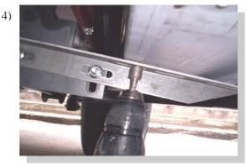
For ABS plastic boards, place on brackets and align on truck. Using self drilling screws attach the board to the brackets.
