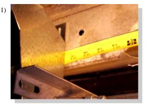
Measure from front wheel well back and make a mark at : Std Cab—10" & 55" Ext Cab—16 1/2", 42"& 60"
