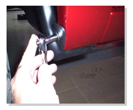
Before installing your running boards remove the small factory stone guard in the front fender well by removing the small screw and then unsnap. Reinstall the screw.
