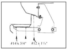
7. Secure GlaStep to body with #12 x 1<sup>1</sup>/<sub>4</sub>" self-drilling screws with rubber washers. Secure step support bracket to bottom of GlaStep using two #14 x 3/4" self-drilling screws per bracket. Tighten all bolts to 18 foot pounds.
