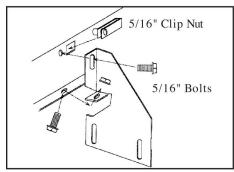
**5.** Find 5/16" holes in pinch weld at 33<sup>1</sup>/<sub>2</sub>" and 64" marks. Secure top of FL83 to rocker panel using 5/16" clip nut in factory locations.
