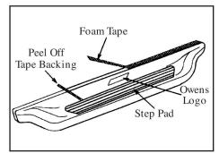
6.Clean surface prior to attaching tape and step pads with denatured alcohol. Apply foam tape to top lip of board. Position step pad on stepping surface. Peel off tape backing starting with rear strip. Keep pad in position, peel off backing then apply pressure to top of pad to stick tape to board. Continue above steps for all tape strips.
