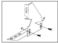
**4.** Assemble FL83 to 3124F using two 5/16" nuts and bolts. **Do not tighten at this time.**
