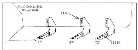
**3. Measure** from front wheel well, back to locations shown above. Mark these bracket location centers. Note: Steel plates have been inserted under fiberglass to mount brackets securely using self-drilling screws.
