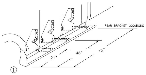
MEASURE FROM FRONT WHEEL WELL TO BRACKET LOATIONS. THERE ARE FACTORY HOLES AT THESE LOCATIONS
