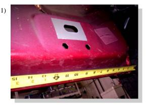
Measure from front wheel well back and make a mark at : Std Cab— 10" & 55" Quad Cab—10", 35", 55" & 66" Crew Cab—10", 35", 55" & 76"
