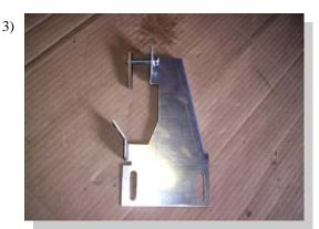
Assemble brackets as shown using one long 5/16" bolt and steel retaining nut. (FL146 shown)
