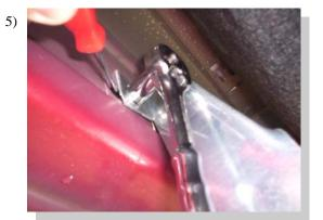
It may be necessary to use a small screw driver to hold against the retaining nut to keep it from turning while tightening the bolt.
