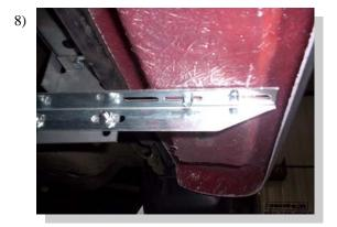
Place the board on the brackets and align up on the vehicle. There is a driver and a passenger side board. Attach to the brackets using #14 X 3/4" long self drilling screws.
