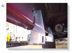
Attach brackets to vehicle by inserting the retaining nut in the factory obround hole and using one 5/16" bolt and nut through the pinch weld. Use the FL145 brackets in the forward locations and the FL146 In the rear most location. (No FL146 is used or included for Std cab models).
