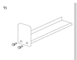
Attach the stone guard to the board with 3/8" self threading bolts.
