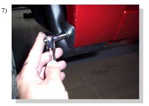
Remove the small factory stone guard in the front fender well by removing the small screw and then unsnap. <u>Reinstall</u> <u>the screw.</u>
