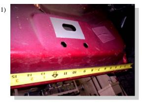
Measure from front wheel well back and make a mark at : Std Cab— 10" & 55" Quad Cab—35", 55" & 66" Crew Cab—35", 55" & 76"
