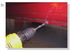
At each of the locations from step one, drill a 23/64" hole through the pinch weld.
