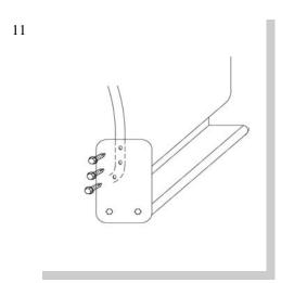
Level board and attach stone guard to vehicle using the sheet metal screws that are included. Tighten all bolts on brackets and repeat for opposite side.
