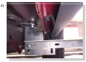
Attach angle support (3124F) to FL122 using 5/16" bolts and nuts. Snug but do not tighten at this time
