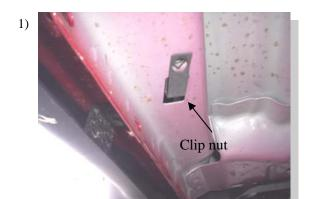
Insert clip nut as shown in factory holes at 15", 38" and 61" on underside of vehicle.
