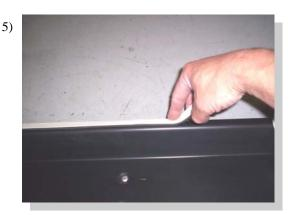
Apply foam tape to the top edge of the running board. Remove the white protective paper before attaching to vehicle.
