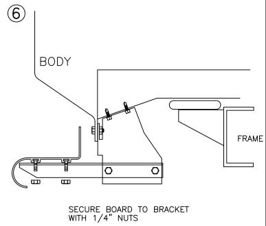
FOR PLASTIC BOARDS, APPLY FOAM TAPE AND STEP TREAD TO BOARD. ATTACH THE BOARD TO THE BRACKETS WITH SELF DRILLING SCREWS.
