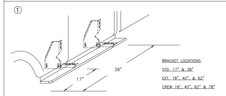
MEASURE FROM FRONT WHEEL WELL TO BRACKET LOCATION MARK THIS DIMENSION ON THE PINCH WELD
