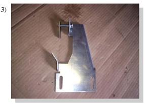
Assemble brackets as shown using one long 5/16" bolt and steel retaining nut. (FL143 shown)
