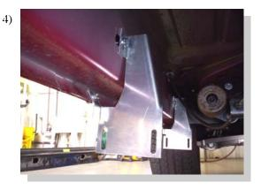
Attach brackets to vehicle by inserting the retaining nut in the factory obround hole and using one 5/16" bolt and nut through the pinch weld. Use the FL142 brackets in the forward locations and the FL143 In the rear most location. (No FL143 is used or included for Std cab models).
