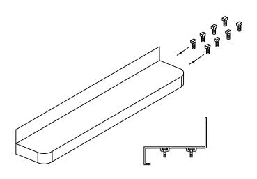
SLIDE ONE 1/4" X 5/8" SQUARE HEAD SCREWS INTO EACH TRACK FOR EACH BRACKET.
