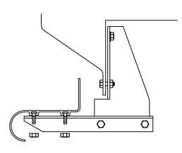
SECURE BOARD TO BRACKET WITH 1/4" NUTS
