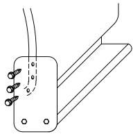
SCREW THROUGH STONE GUARD INTO FENDERWELL LIP USING #14 BY 3/4 SELF DRILLING SCREWS, MAKE SURE YOU DRILL INTO METAL
